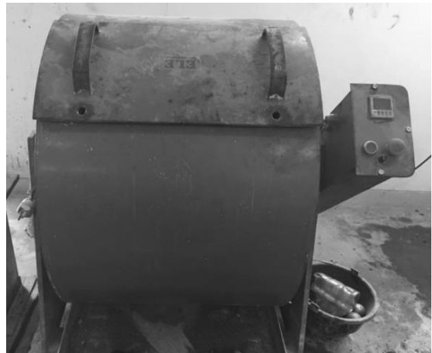
Fig. 2 Los Angeles machine for abrasion test
