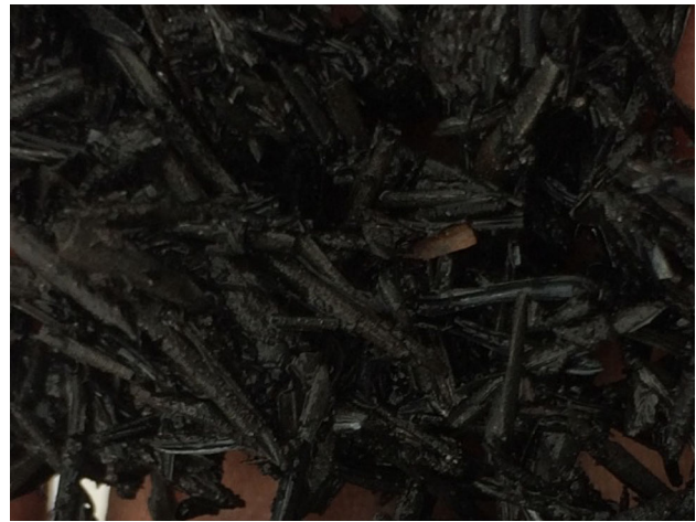
Fig. 1 Residual NRHA after burning process
