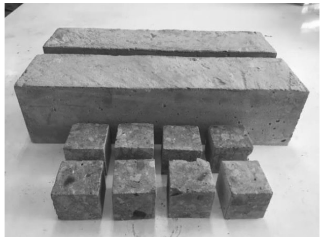
Fig. 3 Specimens for abrasion testing
